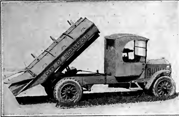
THE REAR COVERS OPEN AUTOMATICALLY
